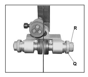
The rear guide blocks should be set so that they are approximately 3 mm behind the blade. They will only come into contact with the blade as the work-piece is being cut.
