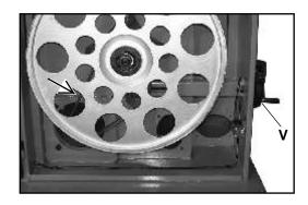
Rotate the belt tension handwheel  $(\mathbf{V})$  to adjust the V-belt tension.
