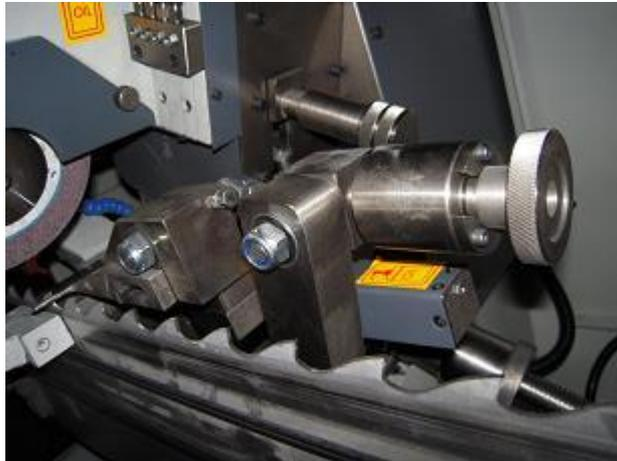
Third adjust the tooth height arm and touch the blade.
