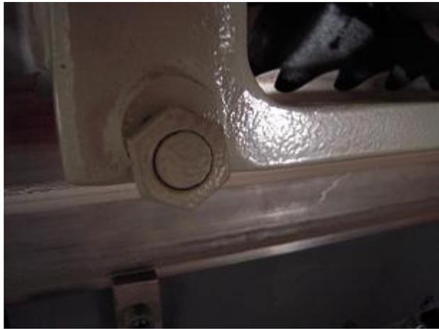
By adjusting the nut on the Picture above, the clamping pressure can be increased by turning in CW direction.
