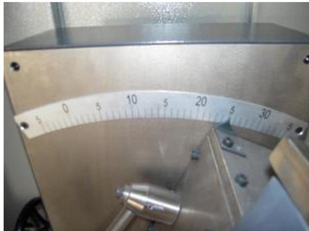
In order to adjust the hook (beta) angle use the wheel below.
