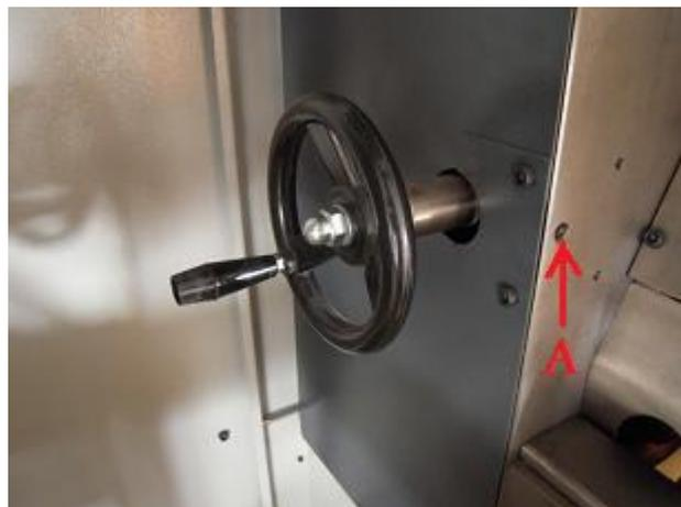
Unlock/lock the screw “A” before/after adjusting the Hook angle.
