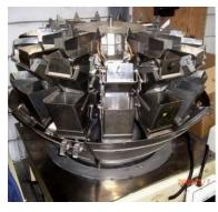
**Ishida CCW-S 211**, 14 heads, 15-1000g, anti-spill (leakproof buckets) '90
