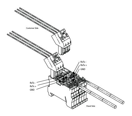
**IMPORTANT:** The plugged termination ensures that the connections are made simultaneously. Failure to attach the cables this way may cause damage to the controller.
