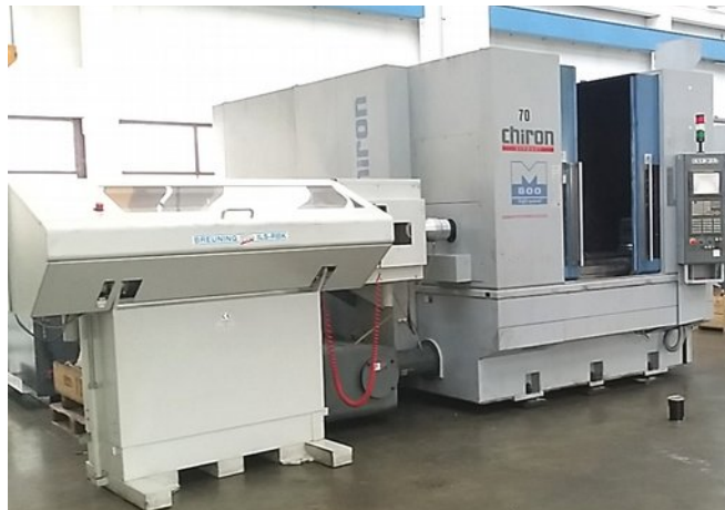
5-axis vertical machining center (milling + turning from bar)
