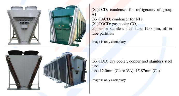
and to units with switching and control components installed – wired or unwired - or with deviations from the standard (X-...).
