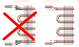
In access lines, a fixed point must be provided at a distance of max. 500mm from the unit connection.
