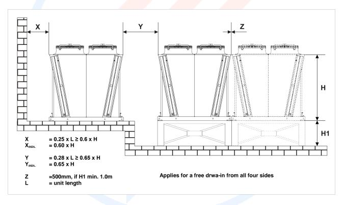
In some circumstances, the lengthwise offset of the units can permit a smaller distance.
