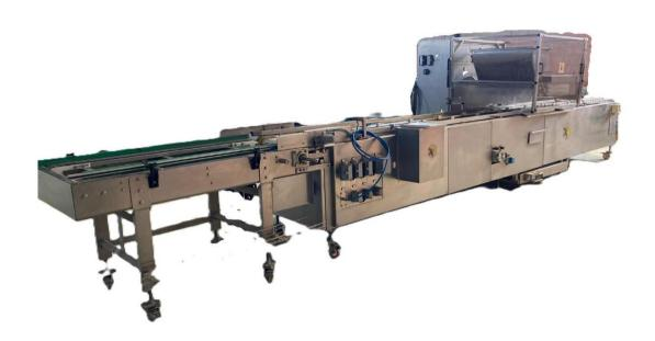
CUP-CAKE-Dosing-Line Line suitable for the production of round CUP-CAKES Ø 45 mm – 90 mm, and small Cakes (Muffins, Magdalenas, Cake-Donuts, Mini-Cake Donuts, Minicakes, Cakebars etc.) arranged on trays of 400x600 mm with 6 x 9 cavities.
